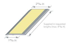
Aluminium floor profile which has been specifically designed to be laid on uneven floor surfaces so that escape route boundaries can clearly be identified in an emergency situation and/or in the event of power failure.
